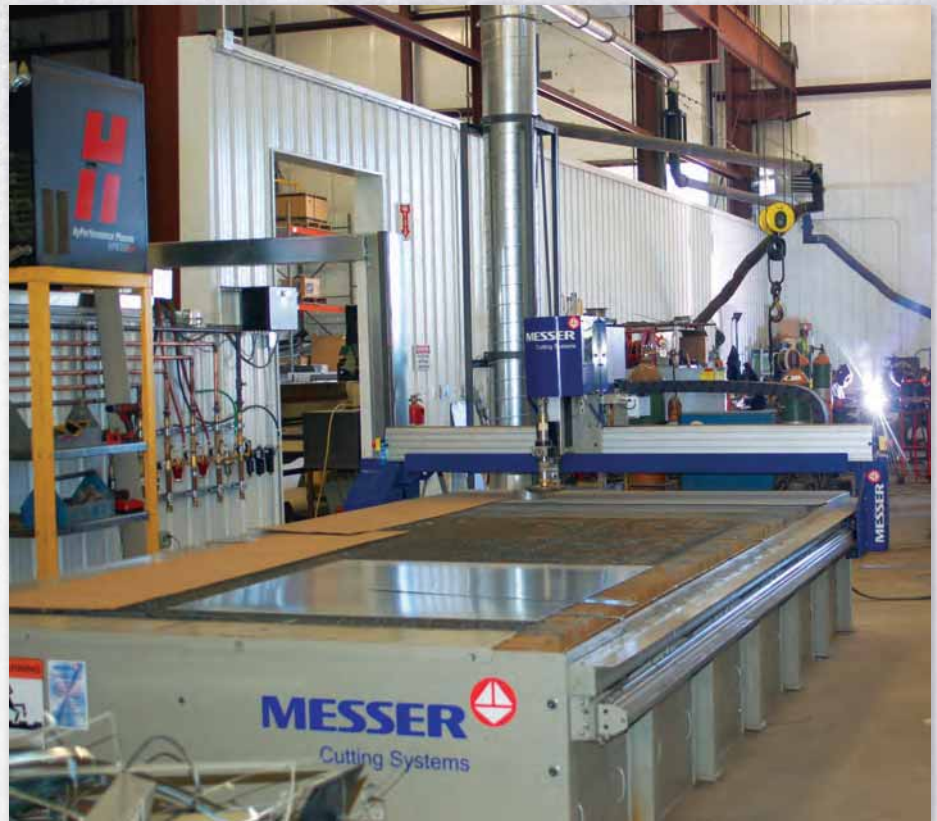
A plasma cutting table is among the new pieces of equipment now in place in A.W. Kuettel & Sons' fabricating shop at its new Airpark location. Note the welder at work in the background.
