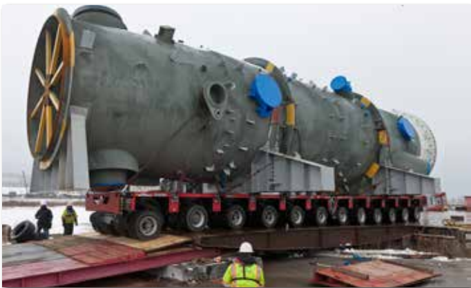
A 187-ton regenerator is off-loaded from the Nickelena Dec. 12
