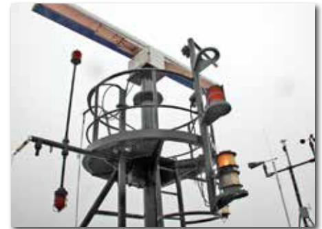
Forward mast and long-range radar antenna. The ship also has a short-range unit.
