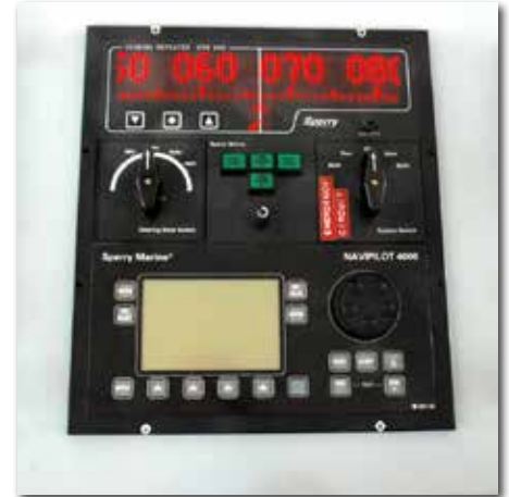
The Sperry Navplot 4000 steering stand on the Hon. James L. Oberstar is tied to the ship's gyrocompass.
