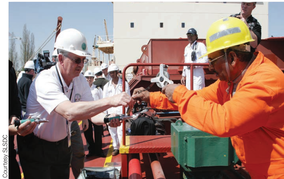
An example of how the binational inspection program works. Former SLSDC Marine Inspector Terry Jordan uses a refractometer to test the salinity of ballast water aboard the Federal Kivalina as the ship enters the St. Lawrence Seaway in Montreal.
