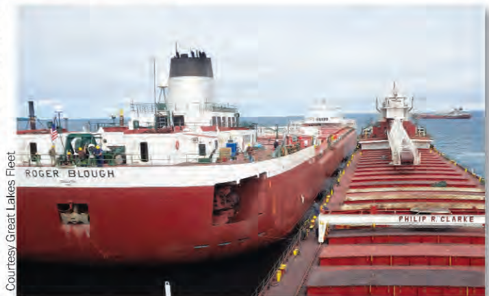
Pellets from the Blough unloading into the Clarke . The 'shuttle boom' on the Blough will not reach high enough to fill trunk hatches on the Anderson or the Clarke , requiring a multi-phase lightering process from the Blough to the Clarke to the Anderson to unload all 45,000-plus tons.
