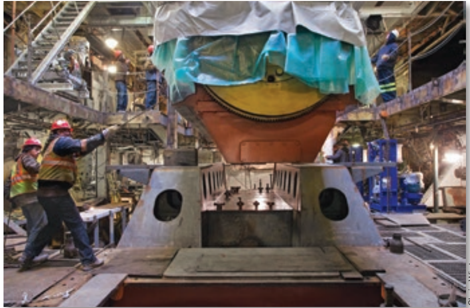
Installation of the new main engine in the John G. Munson
