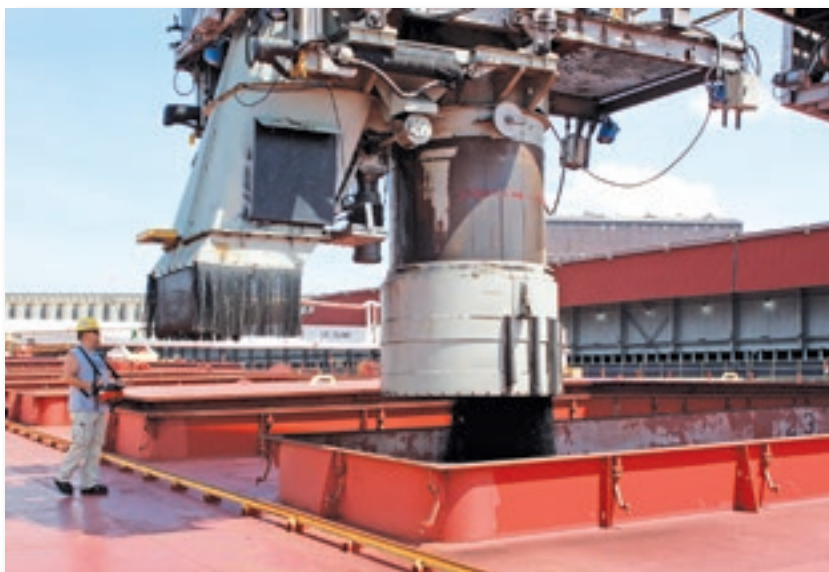
John Rochon, shiploader operator at the Superior Midwest Energy Terminal, loads coal via remote control from the facility's conveyor system into cargo holds on the St. Clair . Coal at that facility can be loaded at a rate of up to 11,500 tons per hour.
