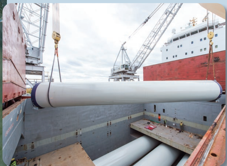
Left: BBC Mississippi arriving Oct. 15, 2020, from India with wind turbine blades and tower sections. Above: BBC Mississippi discharging wind tower components and blades.
