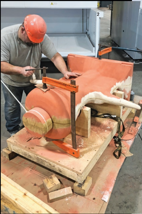
An employee at the foundry glues together part of the mold core. The core is made of zircon sand and resin. This combination helps keep the bollard core hollow, which allows it to be filled with concrete later.
