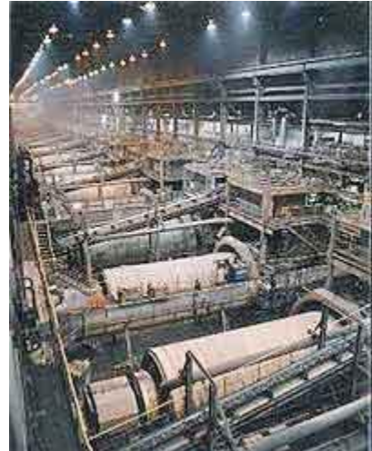
"Pebble mills" are used in taconite processing operations to perform the final grinding of fine particles prior to magnetic separation of high-grade iron ore from waste rock. (Cleveland-Cliffs, Inc., Photo)
