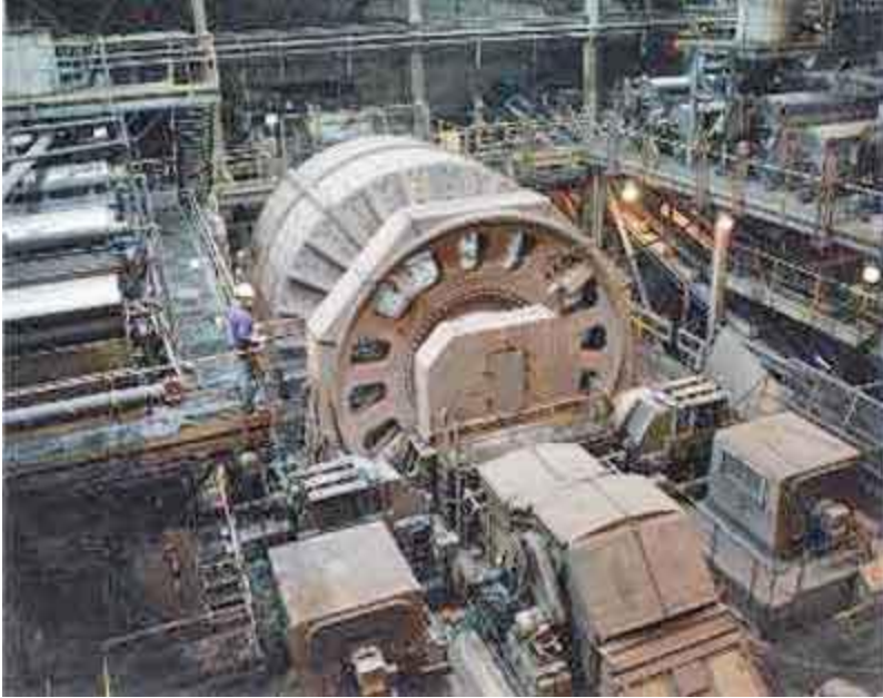
In a modern taconite processing facility, nine-inch diameter crude ore is ground to a powdery consistency in grinding mills of up to 36 feet in diameter. (Cleveland-Cliffs, Inc., Photo)
