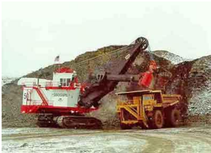
After low-grade iron ore (taconite) is blasted from the ground and broken apart, a gyratory crusher reduces the ore to pieces of about nine inches in diameter and shovels it into 240-ton capacity trucks. (Cleveland-Cliffs, Inc., Photo)
