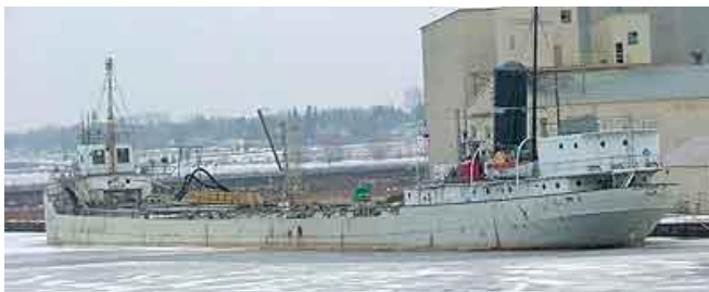
The J. B. Ford, built with a triple expansion engine in 1903, stayed in active service until the 1990s. She now serves as a floating storage facility for Lafarge Cement in Superior, as seen in this January 2004 photo. (Duluth Shipping News Photo)
